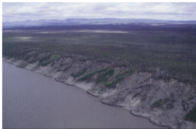
Figure 9. Numerous active-layer detachments along the east bank of the Mackenzie River south of Norman Wells, Northwest Territories, following forest fires in June 1995 (Photo by R. Couture, 1998).
