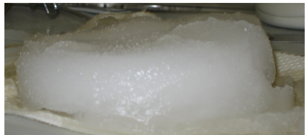
Figure 4: Formed R-11 hydrate
