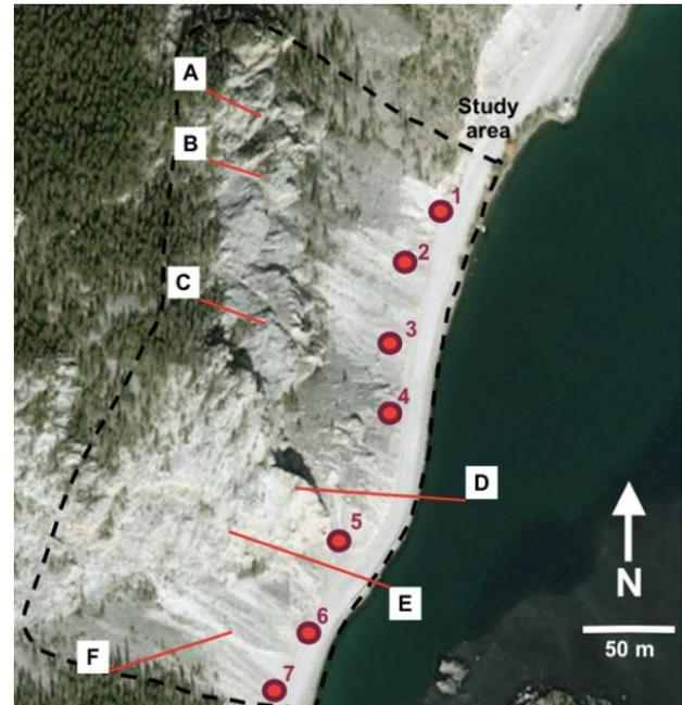
Figure 2. View of the S042 rock slope showing slope sectors A through F for reference through this paper and rock debris window mapping locations 1 through 7
