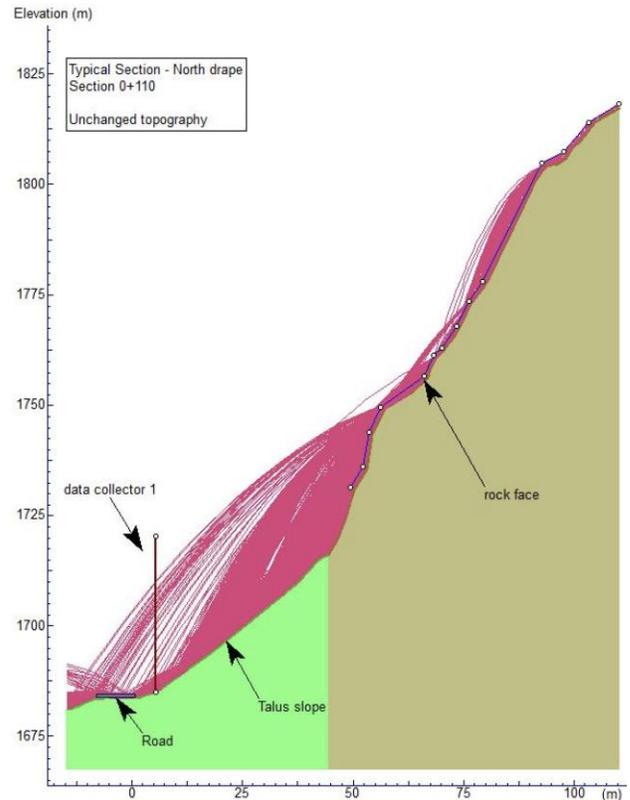
Figure 12. rock fall trajectory model output for existing conditions.
