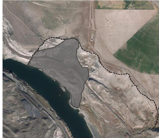
Figure 4: 2015 aerial photo of the Goddard landslide on the east bank of the Thompson River (courtesy of CN rail); shaded area corresponds to the limits of the 1982 reactivation (as per Eshraghian et al. (2007)), dashed line delineates broader extents of an older, possibly ancient landslide feature.
