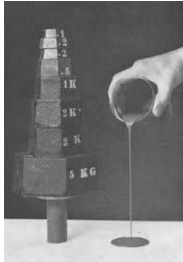
Figure 4: Demonstration of undisturbed and disturbed shear strength of quick clay (Crawford 1963)
