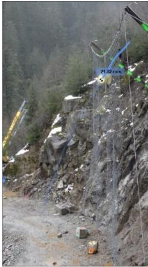
Figure 10: tracking of a block throughout its fall with the software Kinovea.
