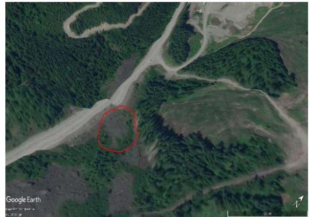
Figure 14: Hope Slide: Deforming area near Highway 3 (red polygon) corresponding to distal limit of coarse debris From: Google Earth.
