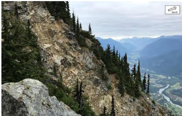
Figure 16. Mount Currie: Field photograph of a disturbed rock mass in area no. 1 of Figure 15. From: BGC Engineering 2018).
