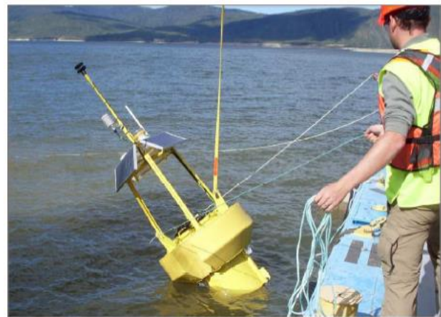
Figure 2. TRIAXYS™ directional wind wave buoy being deployed on Williston Lake reservoir (Photo courtesy - Tetrattech EBA).
