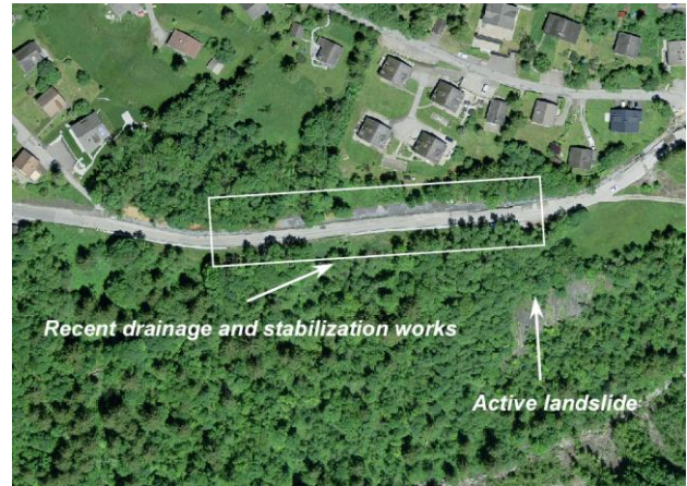
Figure 8: Zone of active landslides that strongly deformed the road, which has been stabilized by important work in 2016 (see the white rectangular box). The location is visible on figure 5 (image from map.geo.admin.ch).
