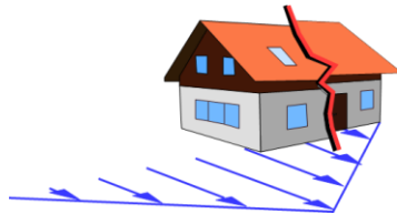
Figure 1: Schematic view of the effect of a differential movement (blue arrows = velocities) on a building.
