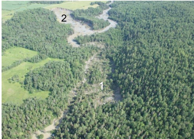
Fig. 1: View of two major retrogressive landslides along the l'Argile river in 2010, Notre-Dame-de-la-Salette. The number one was stopped by rock outcrops.
