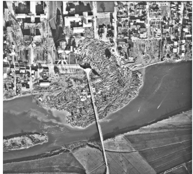
Figure 10. Impact of landslide on community: the November 1955 Nicolet landslide, Québec, a rapid earthflow in Leda Clay. Three people were killed in the landslide which partially destroyed a church complex. The 147-year-old Cathedral of St-Jean-Baptiste, which stood on the edge of the crater, had to be demolished following the landslide. Total damage was estimated to be in the order of $10M (1955)/$71M (2002) (Province of Québec 377-24)
