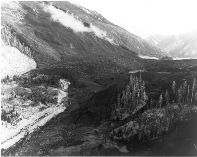
Figure 6. Aerial view of the 1965 Hope Slide, British Columbia shortly after it occurred. The debris filled up the valley bottom and buried BC Highway 3. Note vehicles at bottom left for scale. Four people were killed in the landslide (British Columbia Archives Photograph).
