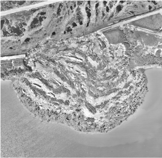
Figure 11. Impact of landslide on highway infrastructure: the 1980 Havre St-Pierre landslide, a retrogressive earthflow in Leda Clay on the north shore of the St. Lawrence, that severed Québec route 138 (AeroPhoto AP8035-087).
