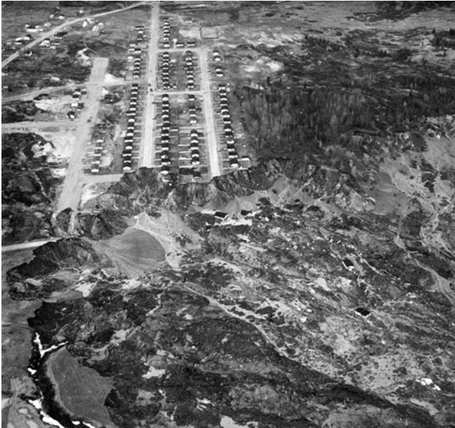
Figure 4. The St-Jean-Vianney landslide, Québec, May 4 th , 1971. Oblique aerial view of the upper part of the landslide scar. Approximately 40 houses were engulfed by retrogression and 31 people died in the Leda Clay earthflow. Some displaced houses are seen in the debris below the scarp. (Canadian Forces Photograph taken on May 7 th , 1971).
