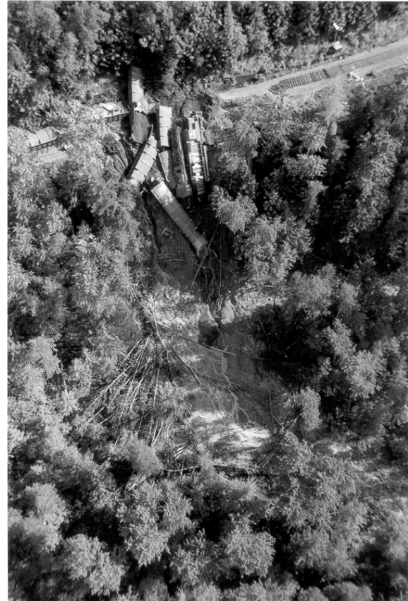
Figure 5. The 1998 failure of a railway fill constructed from glaciolacustrine silt near Creston, British Columbia. The failure, triggered by sustained heavy rainfall, was transformed into an extremely rapid flowslide which swept into the forest below the track up to a distance of 80 m (Transportation Safety Board, 1998).
