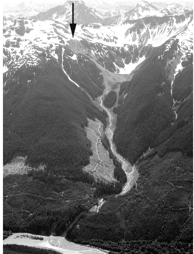
Figure 12. Oblique aerial photograph of 2002 rock avalanche - debris flow in the Coast Mountains, British Columbia. Initial failure volume was ca. 1.4 \times 10^6 \text{ m}^3 . The rock avalanche and debris entrained from the channel travelled 3.7 km from the base of the failed slope and dammed the Zymoetz River (centre bottom left). Source of rock avalanche is indicated by arrow. Just above the river the debris ruptured a natural gas pipeline supplying Terrace, Kitimat and other areas in northwestern British Columbia. Total direct and indirect costs associated with the event are approximately $33.4 M (Schwab et al., 2003).
