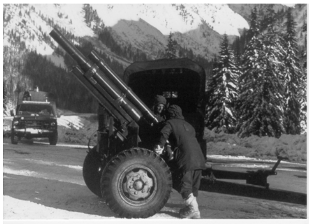
Figure 4: A 105 mm howitzer used to apply explosives for avalanche control at Rogers Pass, BC. C. Stethem photo.
