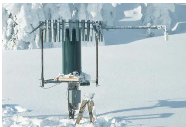
Figure 5: Remote precipitation gauge and ultrasonic snow depth sensor used to monitor snow accumulation during storms. B. Jamieson photo.
