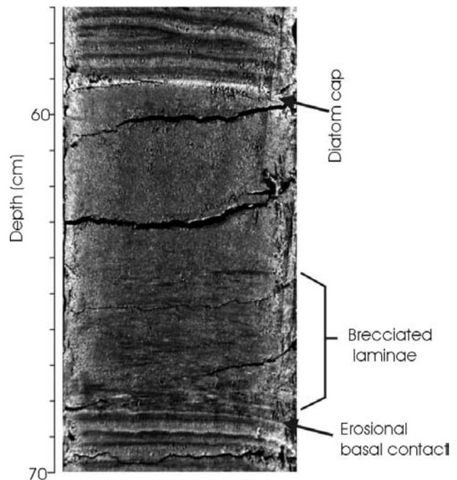
Figure 4. Debris flow deposit showing erosional basal contact, basal zone of brecciated laminae, and diatom cap.
