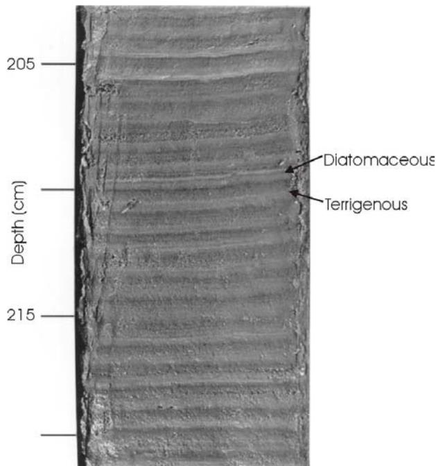
Figure 3. Typical varved sediments. Each couplet comprises a dark lamina of terrigenous sediment (winter layer) and one light, diatom-rich lamina (summer layer).
