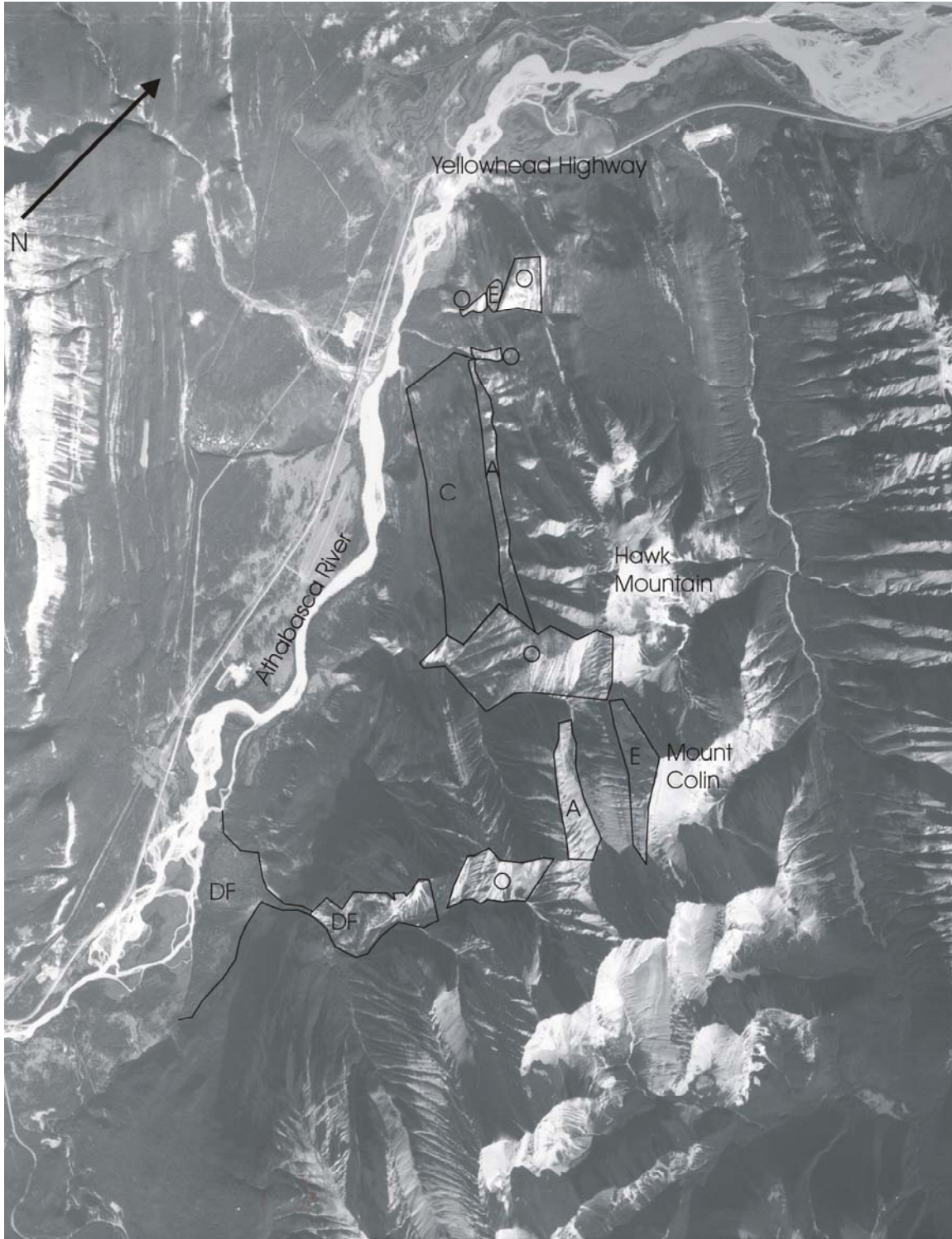
Figure 1 – The west slope of the Colin Range, Jasper National Park, showing areas of exfoliation, E; orthoclinal toppling, O; cataclinal toppling, C, anacinal toppling, A and debris flow deposits, DF, overlain on part of aerial photograph A23025-138, Natural Resources Canada. Scale 1:60 000.
