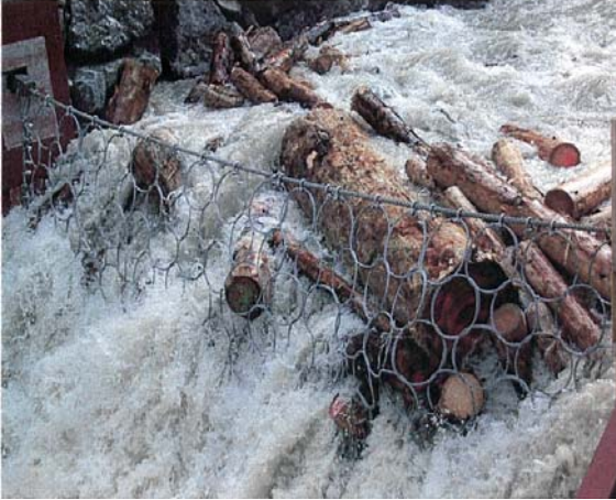
Figure 12. Successful test with woody debris
