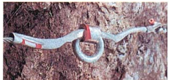
Figure 6. Fully activated pipe braking element
