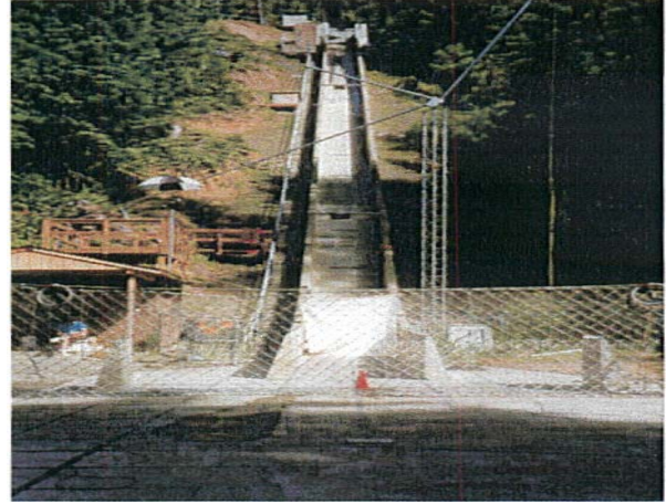
Figure 10. Flexible debris barrier testing at the USGS test flume in Oregon, USA
