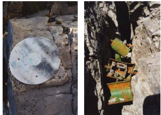
Figure 9: Defaced photogrammetric targets (left) and vandalized Moiré crack gauges (right) observed during the 1999 BGC field investigation (BGC 2000).
