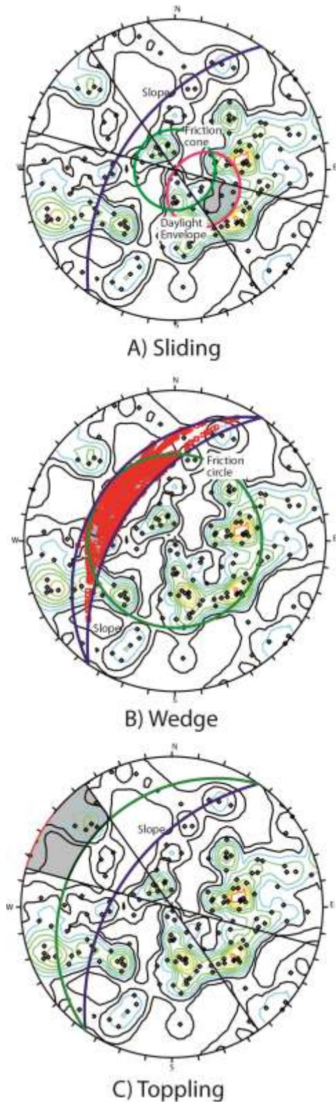
Figure 7: Kinematic analysis using the combined discontinuity dataset. The analysis assumed a slope orientation 50^{\circ}/305^{\circ} (dip/dip direction) and a friction angle of 35^{\circ} .
