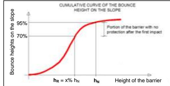
Figure 7. Reduction of the protection level after the first impact: the barrier height is reduced from the nominal value to the residual value.
