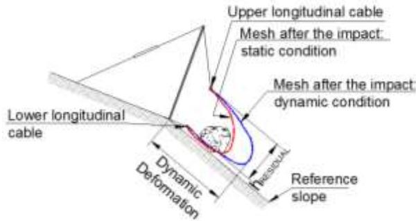
Figure 4. Measurement of the dynamic elongation and the residual height of the barrier, after the impact.
