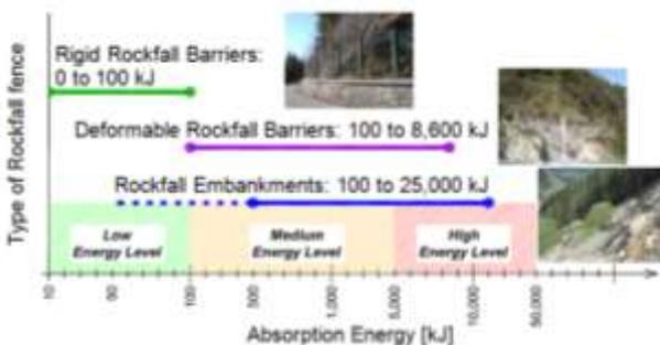
Figure 1. Correlation between the energy level and the type of rockfall barriers (Grimod et al., 2013).
