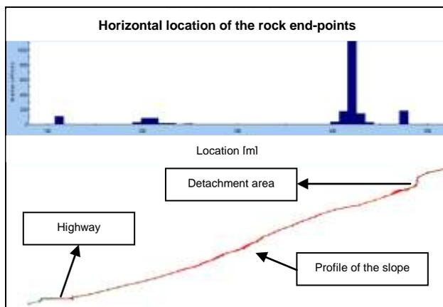
Figure 9. Example of back analysis. Statistical distribution of the horizontal location of the rock end-points; Y-Axis: number of rocks; X-Axis: location in meters (RocFall rel. 4.050).
