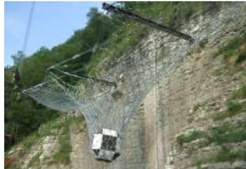
Figure 3. Deformable rockfall barrier tested at the Maximum Energy Level (MEL = 8,600 kJ) according to ETAG 027 (type of fence: RMC 850/A, height = 7.0 m).
