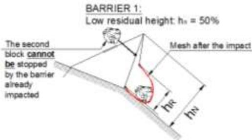
Figure 5. Example of a barrier with a residual height = 50% (classified in Category A according to ETAG 027/2008).
