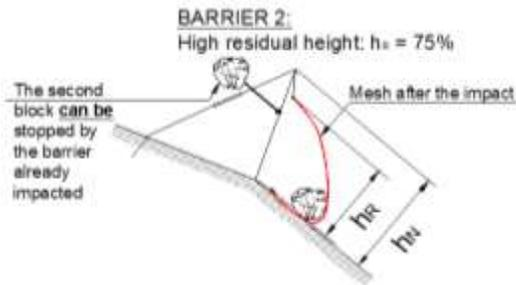
Figure 6. Advantage having a high residual height of the barrier. Example of a barrier with a residual height = 75%, (classified in Category A according to ETAG 027/2008).
