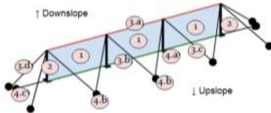
Figure 2. Components of a rockfall barrier.
