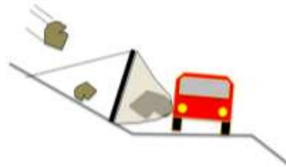
Figure 8. Example of a barrier with an elongation higher than the minimum space available between the fence and the road. The effect of the barrier is neglectable.
