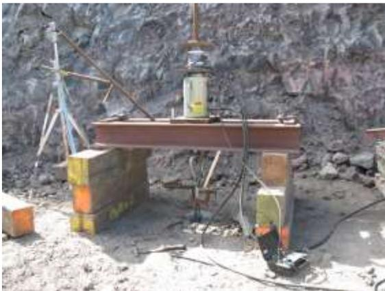
Figure 12. Example of a pull-out test to verify the designed length of the top anchors.
