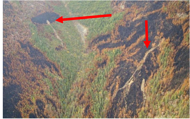
Figure 10. Small landslide activity immediately after the 2009 fire (Photograph P. Lipovsky September 25, 2009).
