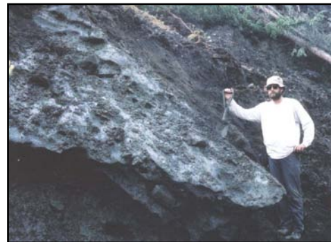
Figure 7. Massive ice found in the lower blocks of the YT Landslide (Photograph by D.J. Hutchinson, August 2004)
