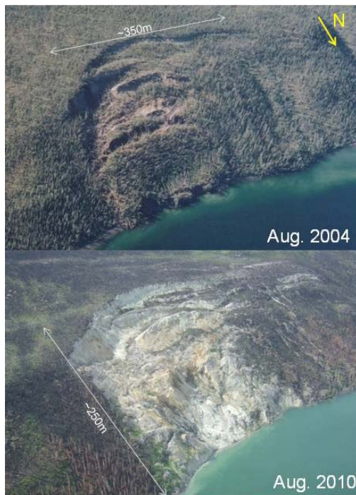
Figure 5. YT Landslide – overview showing significant changes from 2004 (top) and 2010 (bottom) (Photographs by D.J. Hutchinson and J. Koch)
