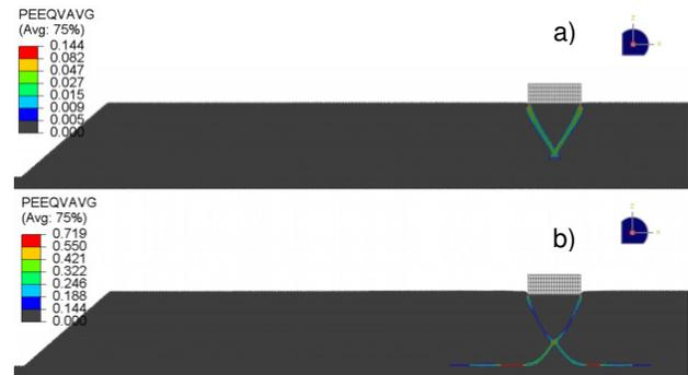
Figure 4. Equivalent plastic shear strain in Case-2 for two vertical displacement of load block: a) 195 mm b) 790 mm
