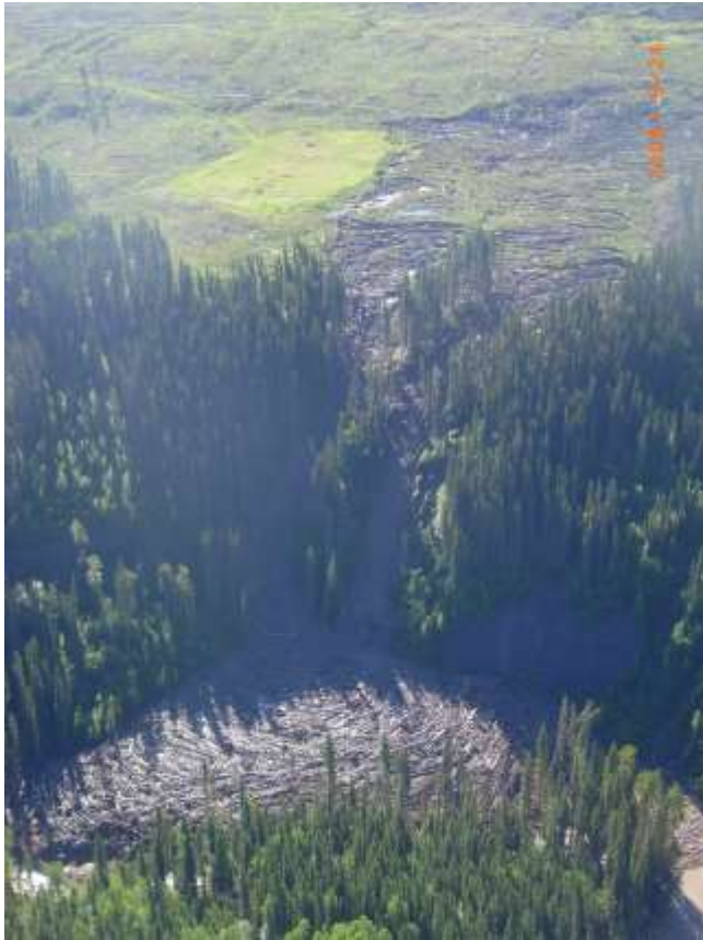
Figure 4. The 2008 Temple Creek landslide. The very wet flow travelled 1 km at 9^\circ .
