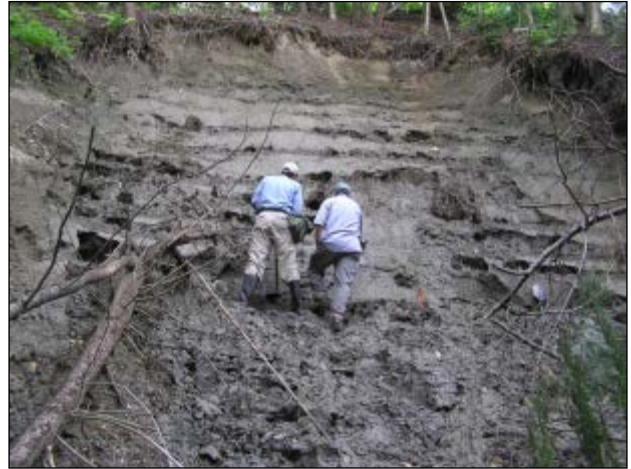
Figure 5. Looking up at top of 2006 slide. Material consists of thick varves composed of 0.46 – 0.76 m layers of fine sand separated by thin silty clay layers (Unit B). Photo courtesy of Jonathan Kim, Vermont Geological Survey.
