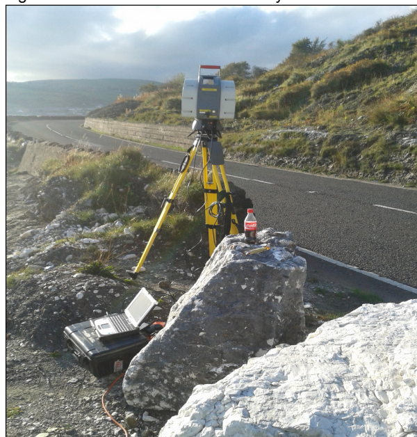
Figure 2. Leica Terrestrial LiDAR scanning of Straidkilly Point, Northern Ireland.
