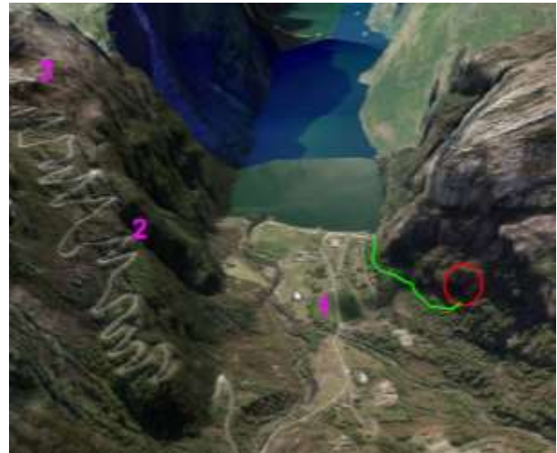
Figure 2. Orthophoto of the Lysefjorden valley. The red circle outlines the tunnel portal, green line is the new road to be constructed, the numbers 1-3 represent TLS and gigapixel imaging locations (imagery from http://www.norgei3d.no/ ).
