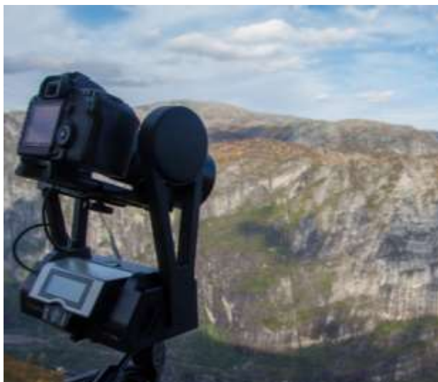
Figure 5. Gigapan robot with Canon 5D MkII and a 135mm f/2.0 L prime lens at data collection location 3 (Figure 2).
