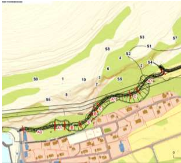
Figure 9. Topographical map with all mapped rockfall hazard locations on the slope face and ranked zones of hazard impact marked along the planned road construction route.
