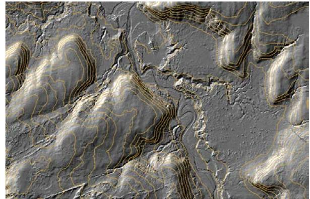
Figure 5 "Bare earth" hillshade LiDAR data with contours.
