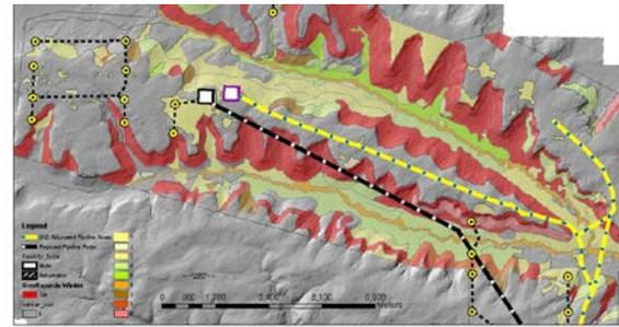
Figure 7 Initial linear infrastructures including pipelines, roads and facilities in black, proposed well pads shown as yellow circles; recommended locations shown in yellow. Red areas (steep slopes, landslides, seepage, exposed bedrock and rock fall) are most problematic in terms of geohazards followed by pink, orange and green (areas with seasonally high water tables).
