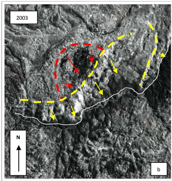
Figures 8a and 8b The main scarp faces (yellow dashed lines) are south facing and are undercut by a creek (white dashed line). The extent of exposed material on these main scarp faces has changed over the time period, with some areas showing signs of revegetation. The red dashed line and arrows show an old but very active sliding unit. The samples for the tree ring analysis were taken in this area.
