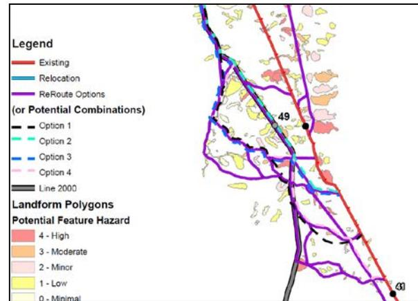
Figure 6 Small section of pipeline route (red) along with a number of potential re-routes.
