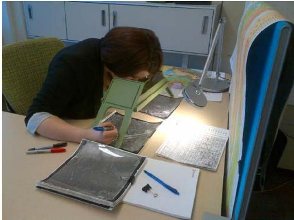
Figure 2 Traditional approach to aerial photograph interpretation using stereoscope and hardcopy aerial photographs.
