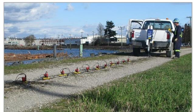
Figure 4. MASW Testing System
