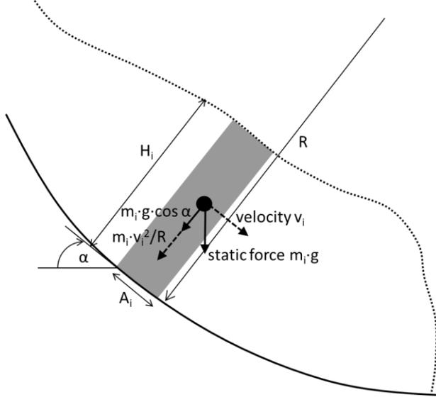
Figure 2. Static and dynamic normal forces acting at base of a sliding element.
