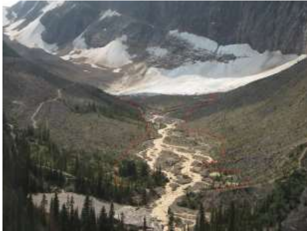
Figure 19 Geometric confinement of potential flood extent in middle reach of valley showing the approximate extent, in red, of a maximum credible flood.
