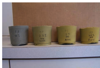
Figure 2. Dyed and un-dyed Grout Samples. Concentrations of dye (by weight of cement) are 0-percent, 2.5-percent, 5-percent, and 7.5-percent, as marked on the samples.
