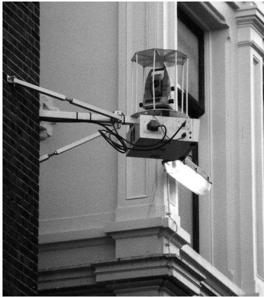
Figure 1. Typical robotic total station
